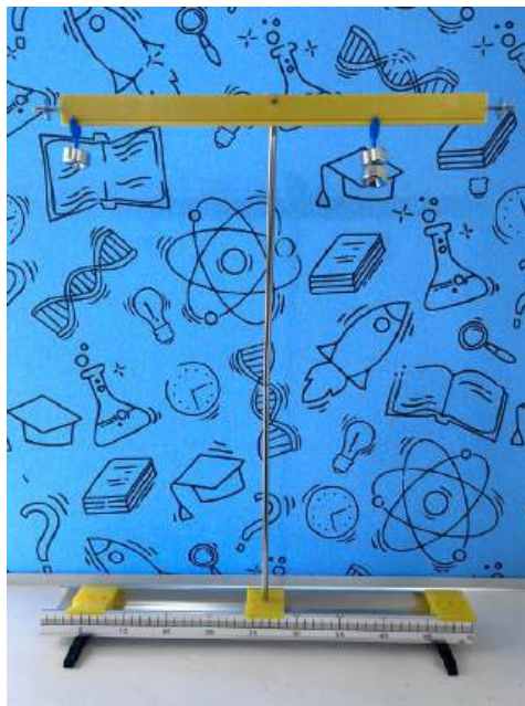
Figure 5. The lever on which the loads are hung
