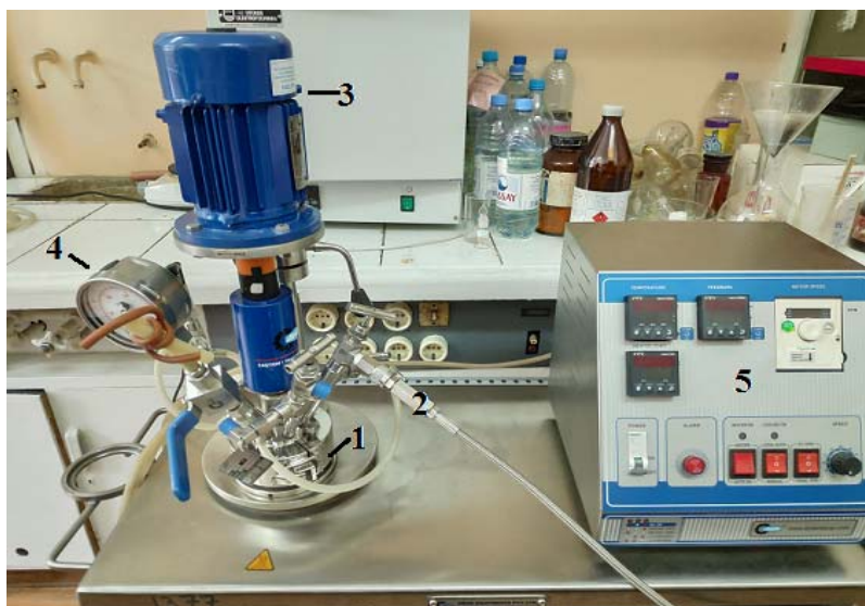
Figure 1 – Oxidation reactor under the oxygen pressure: 1 – reactor; 2 – oxygen supply from the cylinder; 3 – agitator drive; 4 – manometer; 5 – control module
