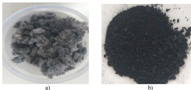
Figure 2 – Samples of textile cord: a- initial, b-carbonized (400°C)
