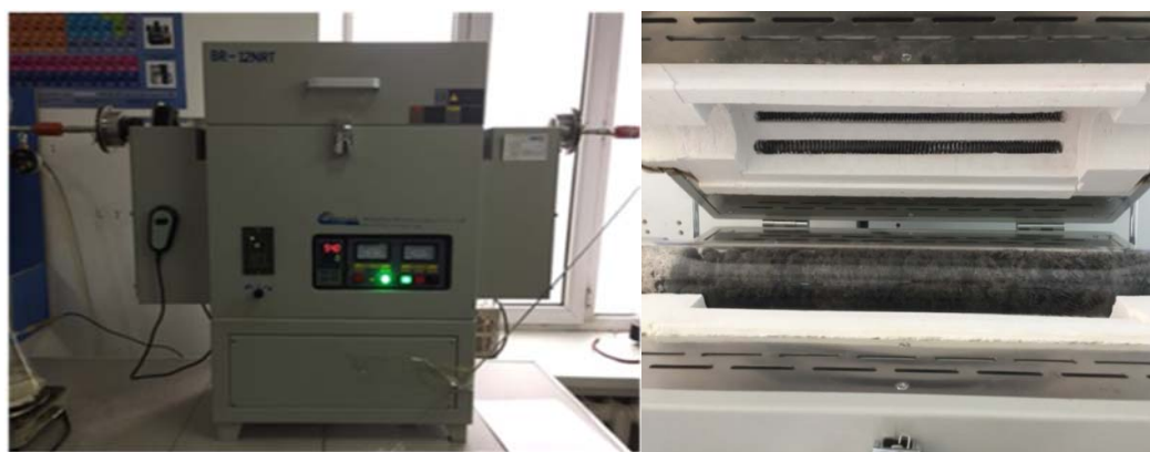
Figure 1 - High-temperature rotary tube furnace BR-12NRT
